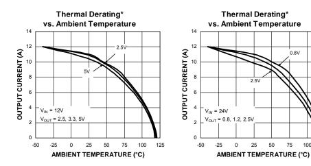
**Die Temperature\***: The temperature measurement was taken at the hottest point on the MIC26901 case mounted on a 5 square inch 4 layer, 0.62", FR-4 PCB with 2oz finish copper weight per layer, see Thermal Measurement section. Actual results will depend upon the size of the PCB, ambient temperature and proximity to other heat emitting components.
