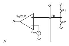
Figure 6. Voltage-Divider Configuration
