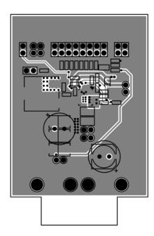
Figure 11. MIC26901 Evaluation Board Mid-Layer 2
