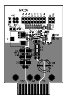
Figure 9. MIC26901 Evaluation Board Top Layer
