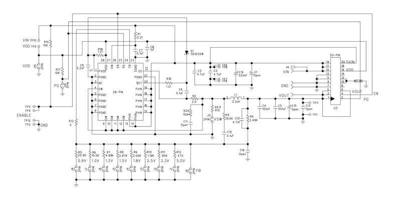
Figure 8. Schematic of MIC26901 Evaluation Board (J11, R13, R15 are for testing purposes)
