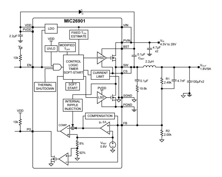
Figure 1. MIC26901 Block Diagram
