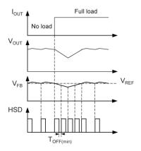
Figure 3. MIC26901 Load Transient Response
