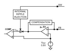
Figure 7. Internal Ripple Injection
