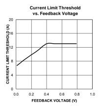
Figure 4. MIC26901 Current-Limit Foldback Characteristic
