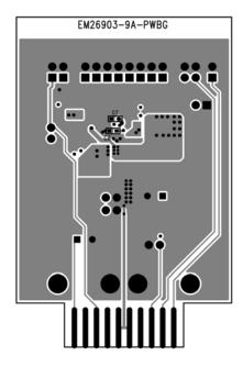
Figure 12. MIC26901 Evaluation Board Bottom Layer
